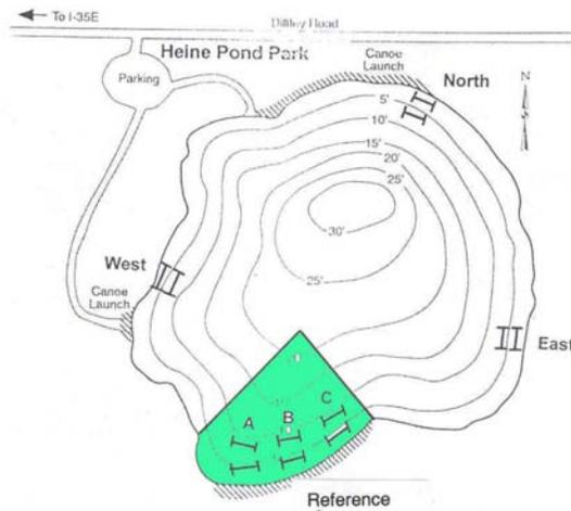
Figure 4. Heine Pond iron treatment map. The shaded area represents the untreated reference area.
